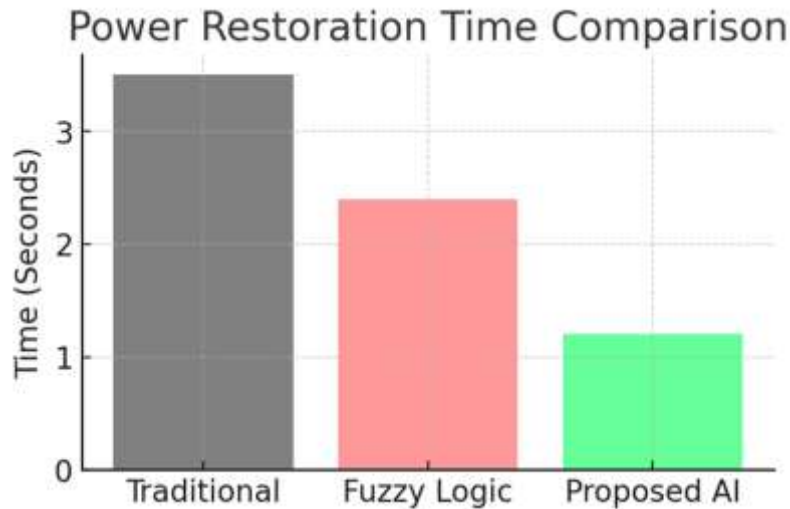
Figure 4. Comparison of Power Restoration Time.
