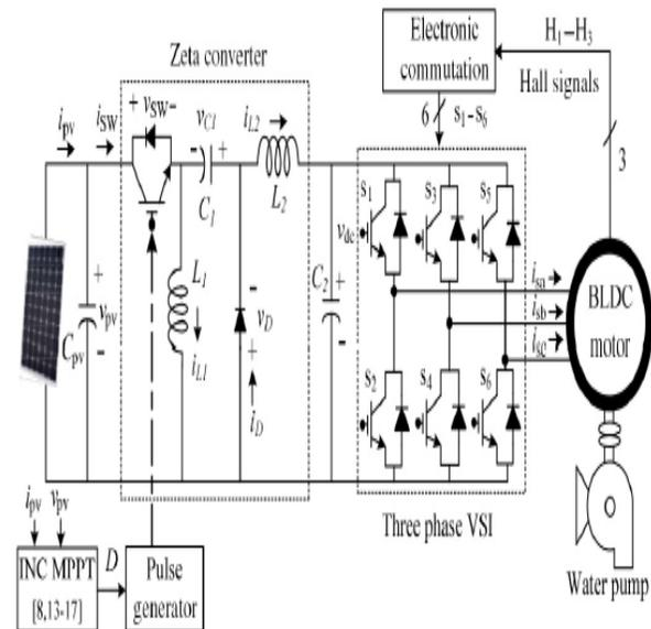
Fig. 3.1. Proposed SPV-zeta converter-fed BLDC motor drive for water pump.
