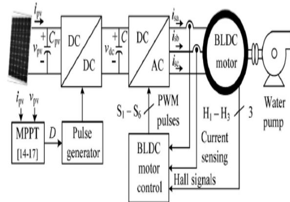
Fig2.1. Conventional SPV-fed BLDC motor-driven water pumping system
