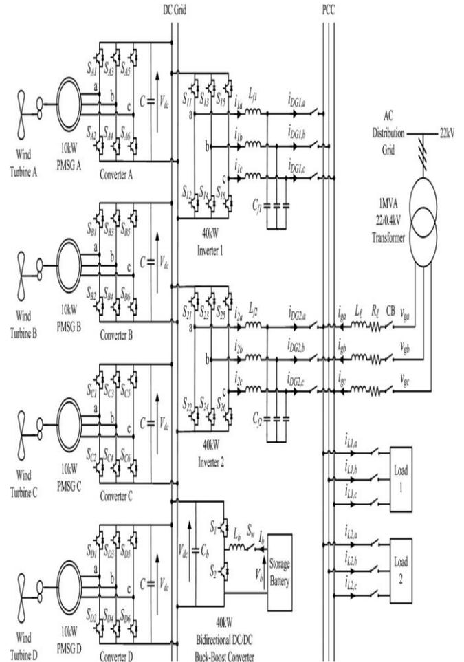
Fig. 2.1 Overall configuration of the proposed dc grid based wind power generation system in a micro grid.
