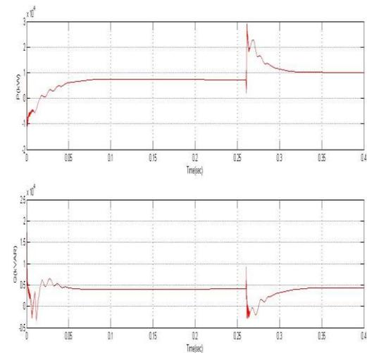
Fig.6.3 REAL (TOP) AND REACTIVE (BOTTOM) POWER DELIVERED BY INVERTER 2.
