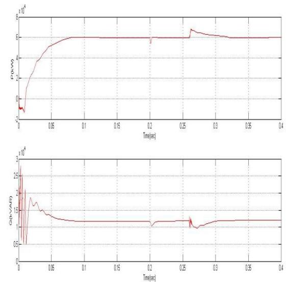
Fig. 6.6. REAL (TOP) AND REACTIVE (BOTTOM) POWER CONSUMED BY THE LOADS.
