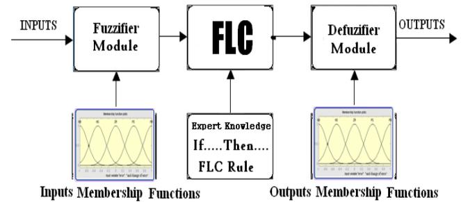
Fig.4.2: Block diagram fuzzy logic Controller.
