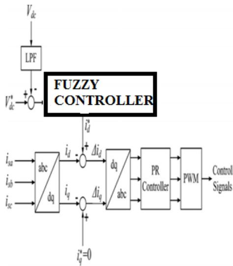
Fig 4.1 Configuration of the proposed controller for the ac/dc converter.
