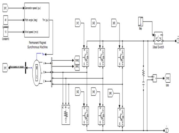
Fig. 6.1 INTRODUCTION OF STEP INPUT RISE AFTER T=0.2 SEC TO AC/DC CONVERTER CONTROL CIRCUIT OF PMSG-A
