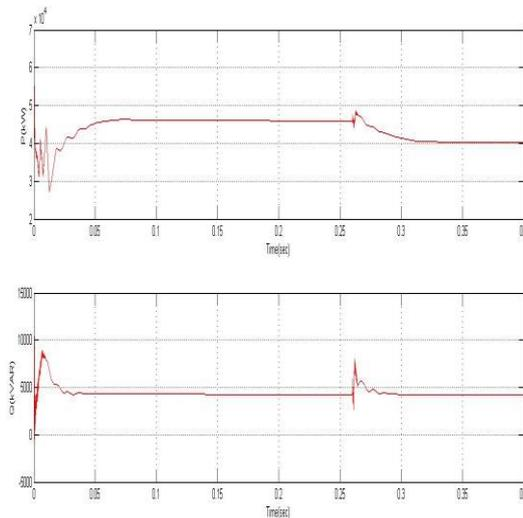
Fig. 6.4 REAL (TOP) AND REACTIVE (BOTTOM) POWER DELIVERED BY THE GRID.
