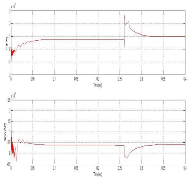
Fig.6.2 REAL (TOP) AND REACTIVE (BOTTOM) POWER DELIVERED BY INVERTER 1.
