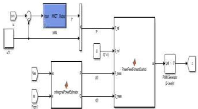
**Fig. 3. ANN-based controller for speed and power regulation.**
