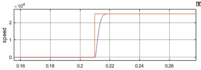
Fig. 9. Reference vs actual speed plot for ramp-up from 0 to 25,000 RPM.
