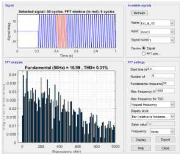
Fig. 10. Harmonic distortion analysis during ramp-up condition.
