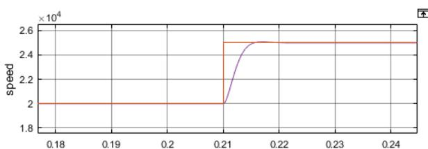
Fig. 11. Reference and actual speed response during step increase from 20,000 to 25,000 RPM.
