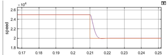
Fig12. Reference and actual speed response during step-down from 25,000 to 20,000 RPM.
