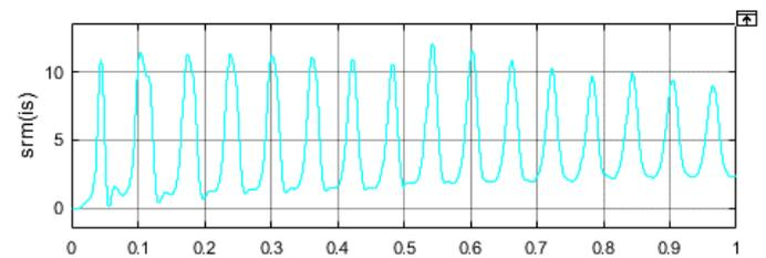
Fig. 7. Motor phase current waveform during steady-state at 20,000 RPM.
