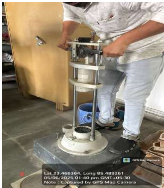
Fig -5: Impact test on aggregates
