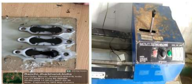
Fig -8: Ductility test on bitumen
