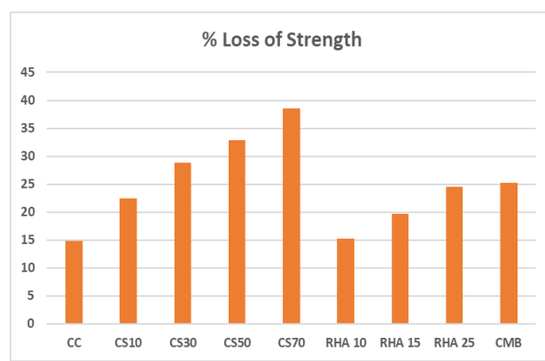
Fig. j: Loss of strength in Acid resistance test
