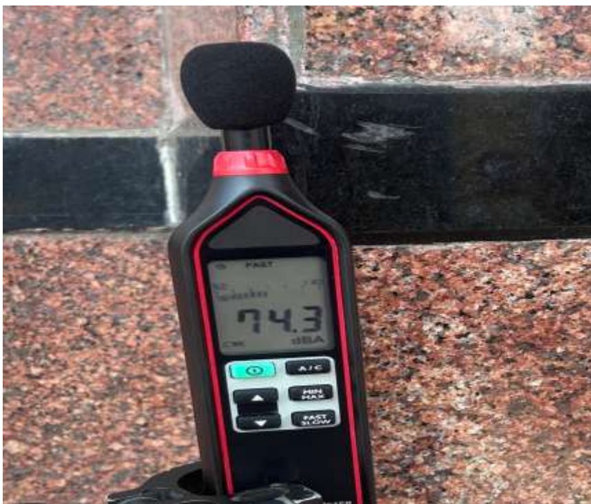
Figure 1: Digital Sound Level Meter used for noise monitoring during field data collection.
