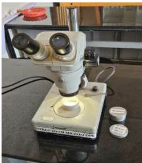
Fig 2. Laboratory setup featuring the Magnus Stereo Zoom Microscope (10x to 40x) utilized for visual identification of isolated microplastics.
