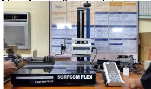
**Figure 3: Surfcom FLEX 50-A-Used for Measuring surface roughness.**
