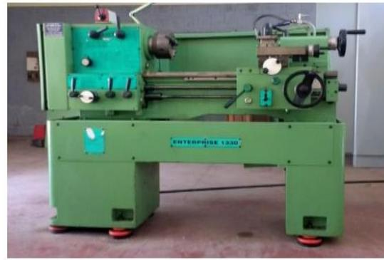
**Figure 1: Automated all geared head lathe.**
