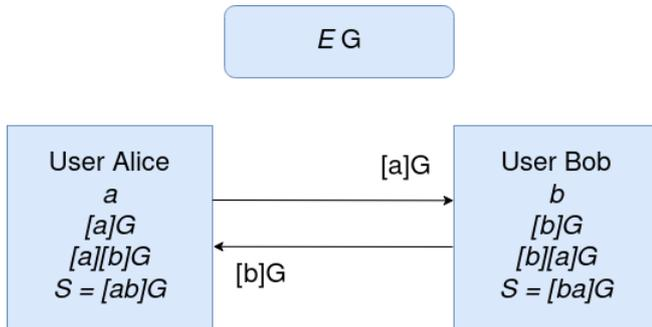
Figure 1: Key exchange in ECC.
