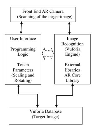
Figure: Data Flow Diagram
