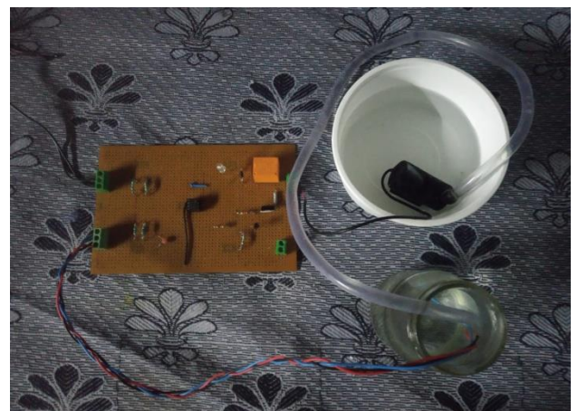
Fig-11: Model of Auto Water pump switcher
