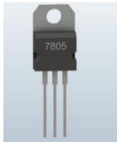
Fig-5: 7805 Voltage Regulator
