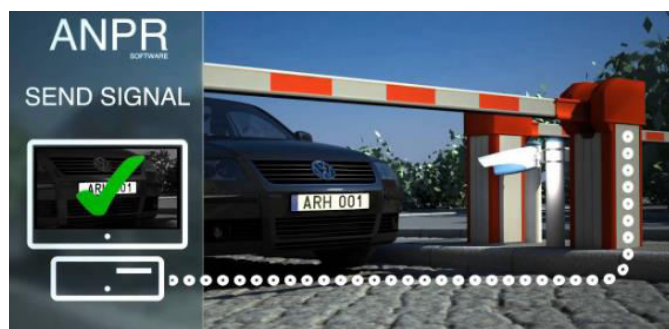
Figure 4: ANPR sending approval signal
