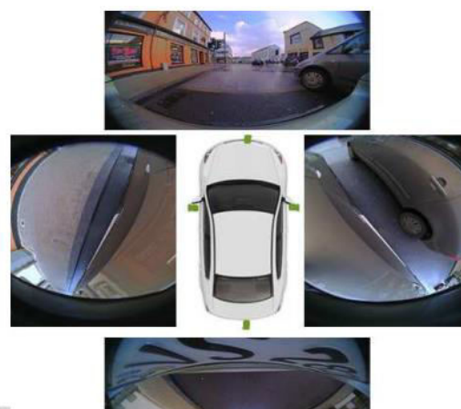
Figure 2: 360-degree view of camera capturing image of a car
