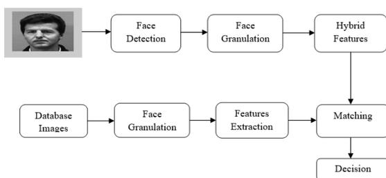
Fig 1.1: Block diagram of the face recognition system
