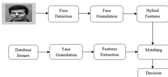
Fig 1.1: Block diagram of the face recognition system
