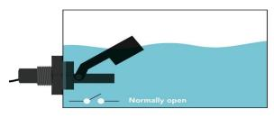
Fig -3: Float Switch Working In Normally Open
