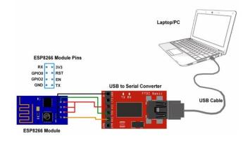
Fig -7: ESP8266 Module Serial Connection with PC
