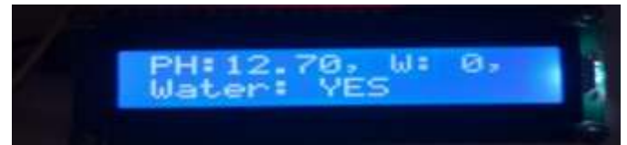
Fig3: LCD Display showing the results of pH values , and presence of water
