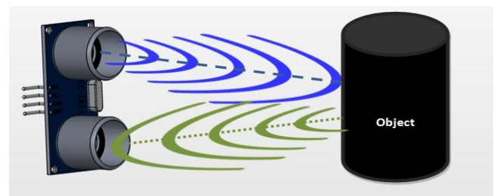
Figure 5- Working of an Ultrasonic Sensor
