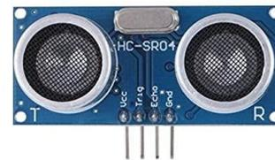
Figure 2: Ultrasonic Sensor
