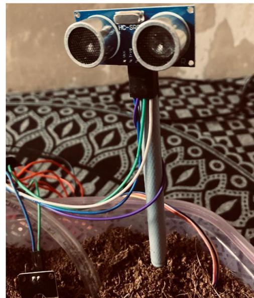
Figure 11: Ultrasonic sensor and water level sensor for deterrent system and sensing the moisture of soil to be displaye
