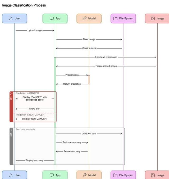
Fig 1 : Sequence Flow Diagram
