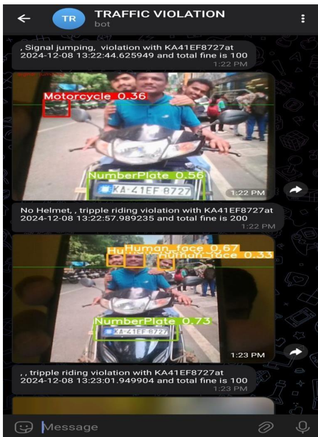
Fig 6 : Message Based Fine Generation for Triple Riding and No Helmet
