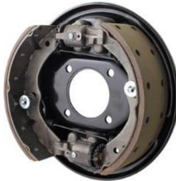
Fig 1.2 Drum Brake
