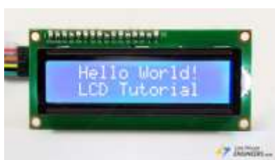
Fig 3: LCD with I2C
