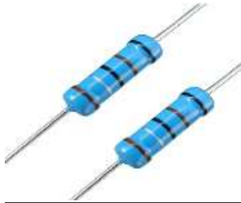
Fig 6: Two resistors of 330 Ohm
