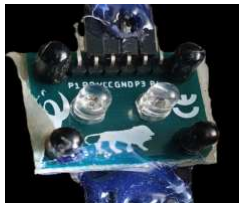
Fig -5: Color Sensor (TCS230)
