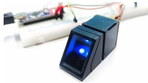
Fig 4: R307 Bio Metric authentication
