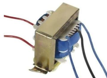
Fig.9 Transformer 12v
