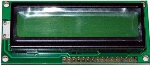
Fig.3 LCD Display
