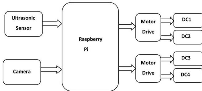
Fig.7: Block diagram
