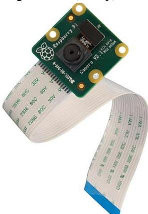
Fig.2: Pi Camera Module
