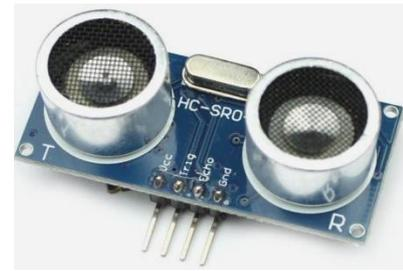
Fig.3: Ultrasonic sensor
