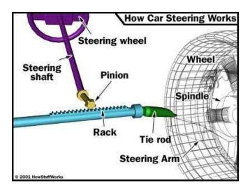
Figure 7 (Working of Steering)
