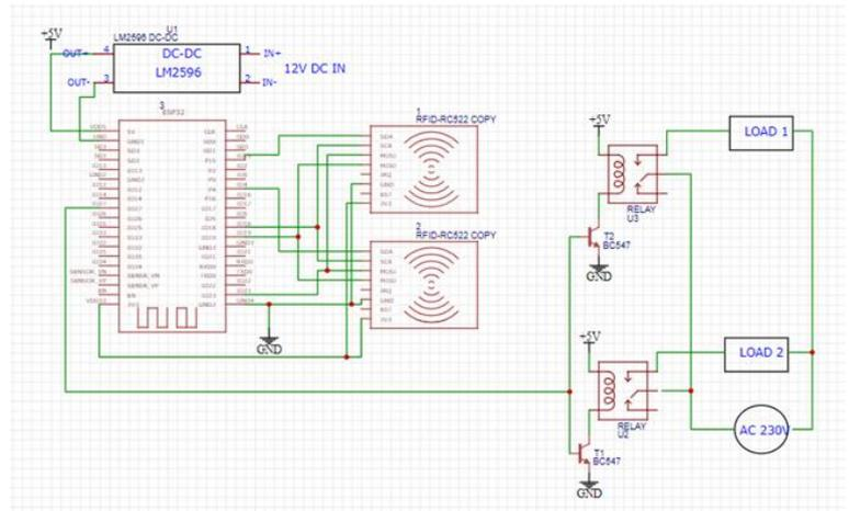
Fig 2: Circuit Diagram of Model
