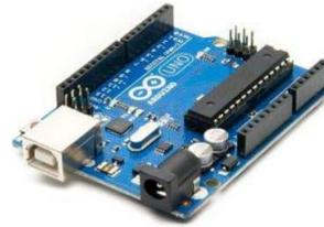
Fig 8. Arduino UNO Board
