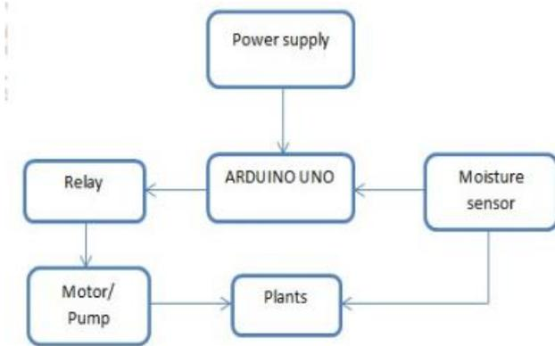
Fig 1. Block diagram of automatic plant watering system.
