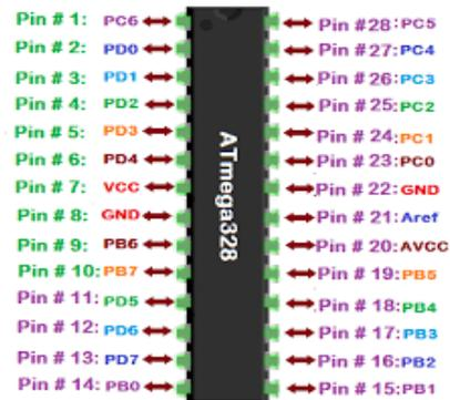
Fig 3. ATmega 328(AVR) pins
