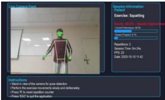
Fig. 2: Example of a rehabilitation exercise captured using a webcam. Pose keypoints are extracted for GCNN-based analysis.
