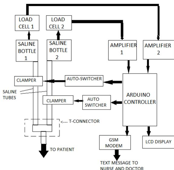
Fig 4: System architecture
