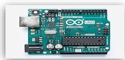
Fig. 3 Arduino Uno Board
