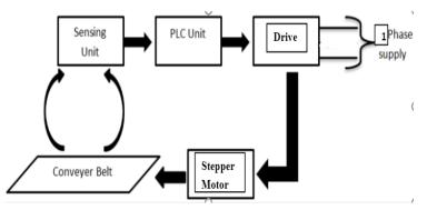
Fig.no. 4 Block Diagram of Working of conveyer belt
