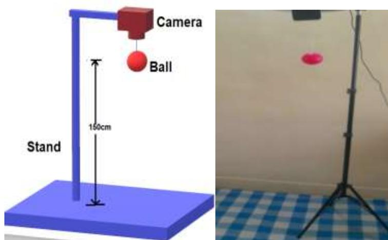
Fig 1. Set up for dropping ball
