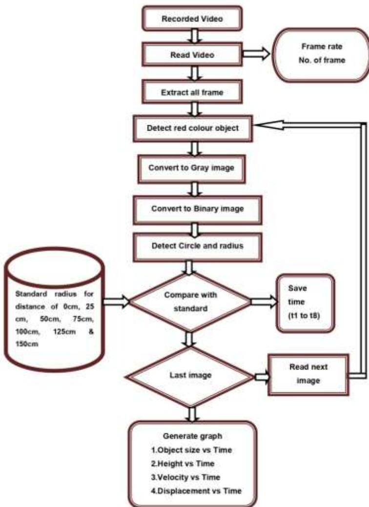
Fig 3 Process Flowchart
