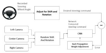
Fig -2: Architecture of the designed model
