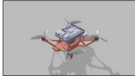
Fig 3. CAD Model with Raspberry Pi 5
