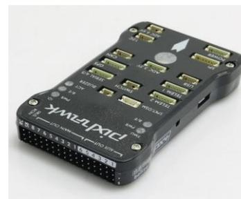
Figure 3.2. Pixhawk flight controller
