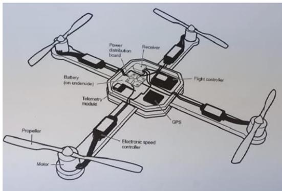
Figure 3.9. Autonomous Drone Architecture
