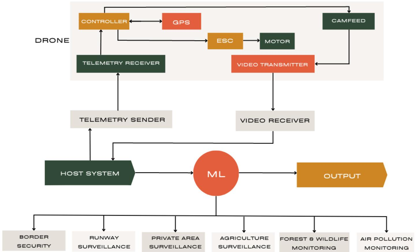
Figure 4.2. Block Diagram
