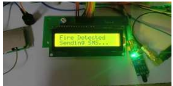
Figure 4: LCD Display when fire Detected
