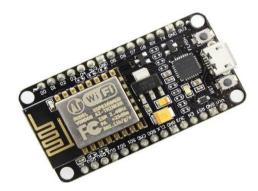
Fig.6.Wifi Module for wireless communication.
