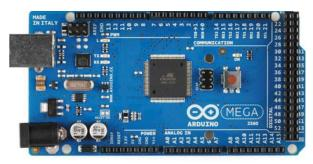
Fig.2. Arduino Mega 2560 for controlling the functions.
