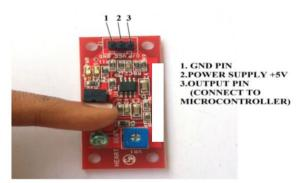
Fig.5. Heartbeat Sensor to check pulse rate
