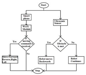
Fig.1. Block Diagram for Proposed System.
