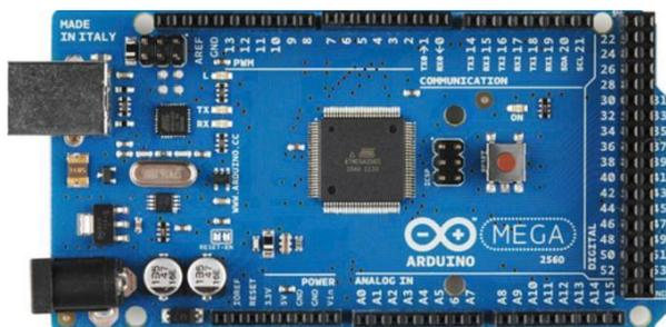
Fig.2. Arduino Mega 2560 for controlling the functions.
