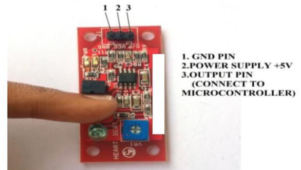
Fig.5. Heartbeat Sensor to check pulse rate
