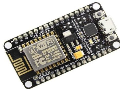
Fig.6. Wifi Module for wireless communication.
