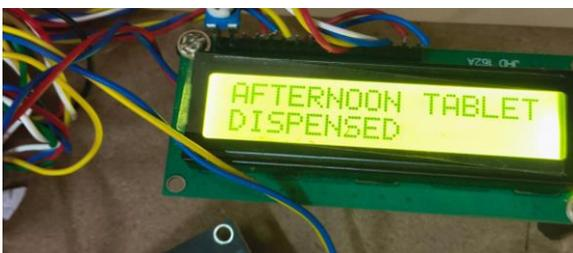
Fig.10.: Display Picture of Afternoon Tablet Dispensary
