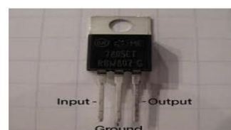
Pin diagram of 7805
