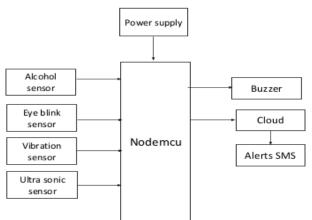
Fig 1: System Architecture
