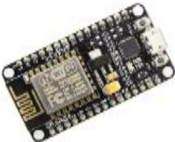
*Fig 2. Nodemcu*
