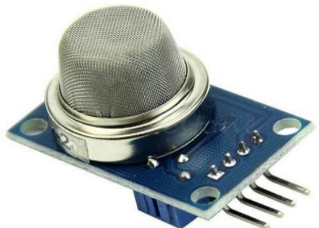
*Fig 5. MQ2 Sensor.*
