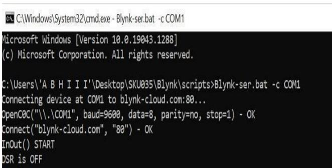
Fig 4: Command for connection of COM Pin
