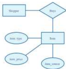
Fig. 3.2. Simplified Entity-Relationship Diagram for the BarterHaven database.
