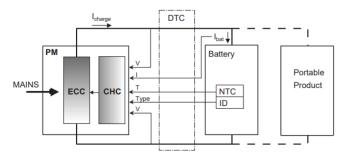
The image represents a battery management system integrated into a Power Module (PM). It efficiently monitors the charging process, hence permitting the proper and safe usage of the battery.
