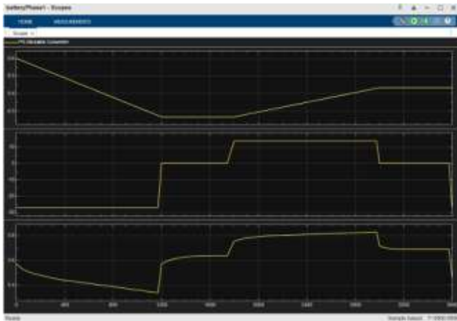
Figure 2. Simulated load current (top) and true vs. estimated SOC (bottom) over a 2-hour trip.
