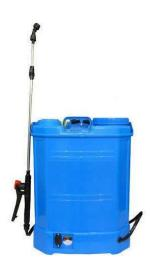
It is operated by a battery which create a pressure difference in which pesticides and liquid is forced through nozzle in fine droplet form. The pressure of this sprayer approximately 7 kg/sq cm. and capacity of storage tank is less than 20 liters.
