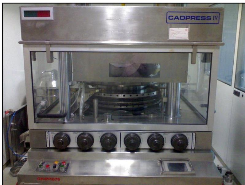
**Figure 8: Cadpress-Bilayer Rotary Machine**
